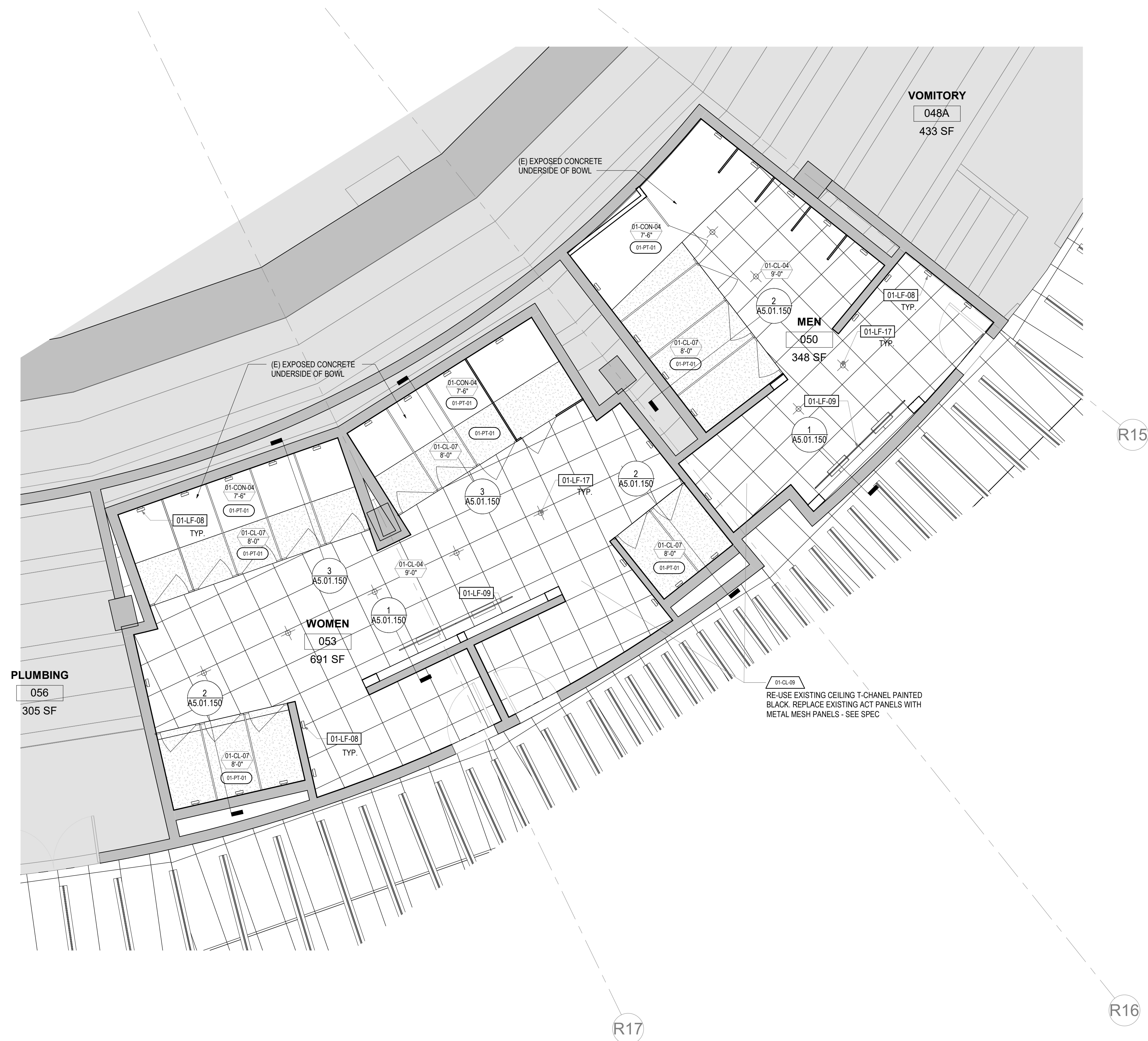
1 ENLARGED RCP - RESTROOM - LEVEL 100 SCALE: 1/4" = 1'-0"
